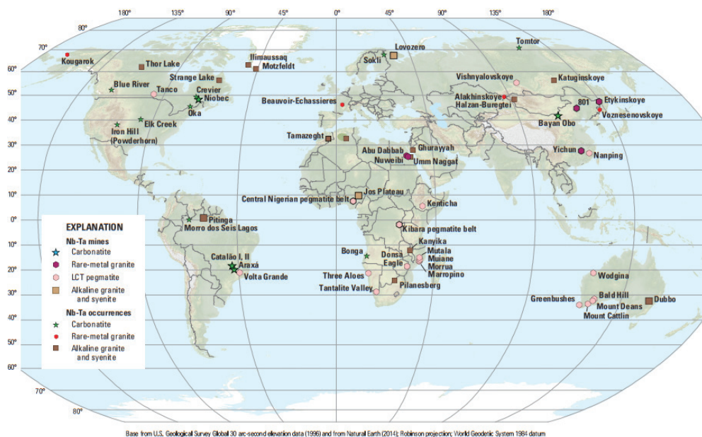
Figure M5. World map showing locations of selected niobium and tantalum mines, deposits, and occurrences, by deposit type. Not all the mines are currently active. LCT, lithium-caesium-tantalum; Nb, niobium; Ta, tantalum
