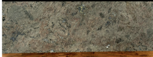
SLM24-057 – Zn-Cu-Pb-Ag Endoskarn at 114.00m.
