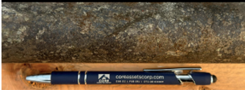
SLM24-061 – Fe-Zn-Cu-Pb-Ag Massive Sulphide at 4.25m.
