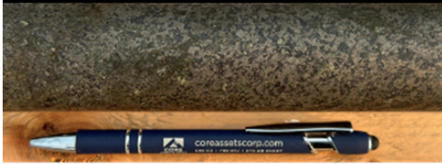
SLM24-061 – Fe-Zn-Cu-Pb-Ag Massive Sulphide at 4.25m.
