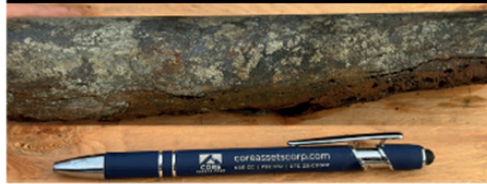
SLM24-057 – Zn-Cu-Pb-Ag Endoskarn at 114.00m.
