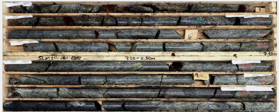
Photograph of the continuous 11.8-metre interval of massive sulphide (sphalerite-pyrrhotite-pyrite +/- chalcopyrite-galena-rich) skarn mineralization in Sulphide City-Whaleback hole SLM24-061. (Source: News-release on August 7, 2024 )
