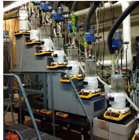
Continuous HCl Leach Pilot
