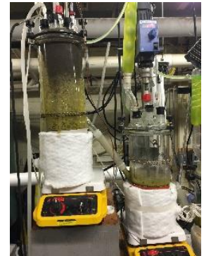
Continuous HCl Leach Pilot
